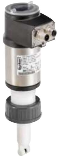
Conductivity transmitter with programmable outputs. Conductivity and temperature output via single or dual analog 4-20 mA. Two transistor outputs are also included. Transmitters are engineered for a wide scope of measuring ranges and can be delivered in 2-wire or 3-wire configurations. Intelligent, integrated, beautiful design fits perfectly with an assortment of easily configured fittings.
